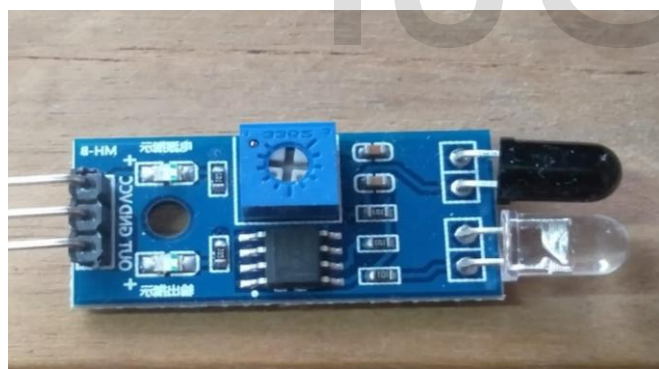
Fig.2 : Infra-Red obstacle detection sensor
